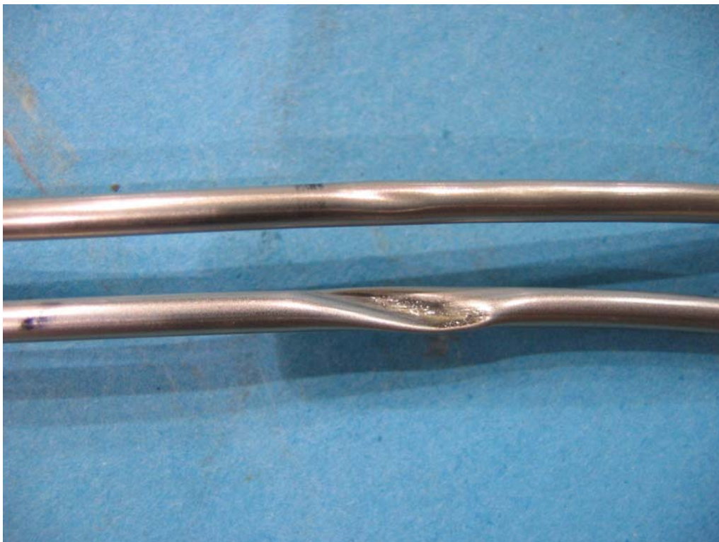
Figure 3b Dissected SS Tubes from Impact Test
