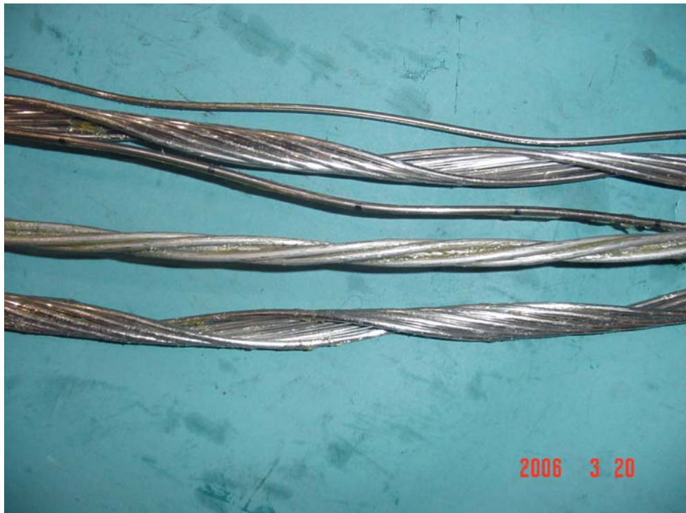
Figure 3b Dissected Components from Aeolian Vibration Test (Under Passive Dead-end)
