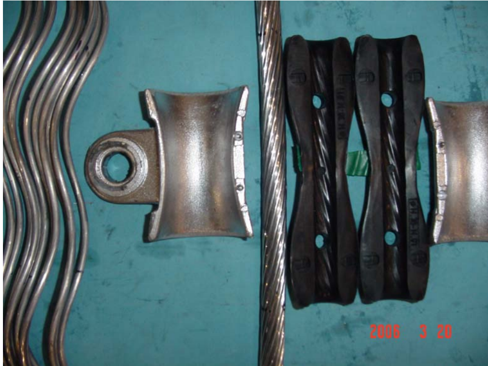
Figure 3c Dissected Components from Aeolian Vibration Test (Suspension)
