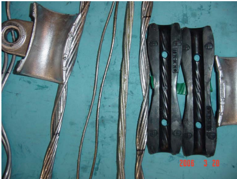
Figure 3d Dissected Components from Aeolian Vibration Test (Suspension)
