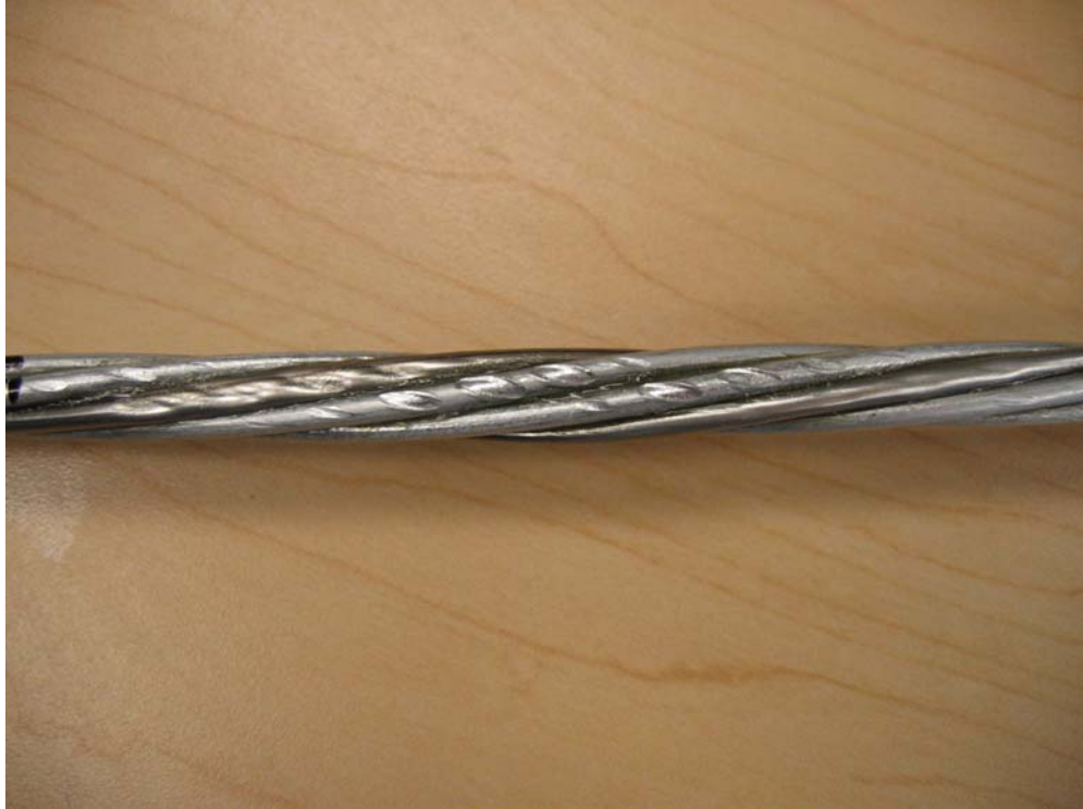
Figure 3a Dissected Sample from Crush test (AA wires removed)
