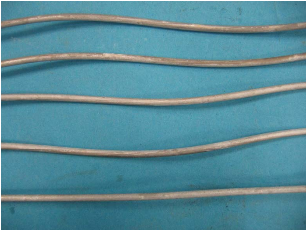
Figure 3d 5 Tested Individual ACS Wire Samples after 1000 hours
