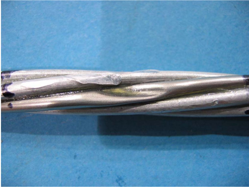
Figure 3a Dissected Sample from Impact Test (AA wires removed)
