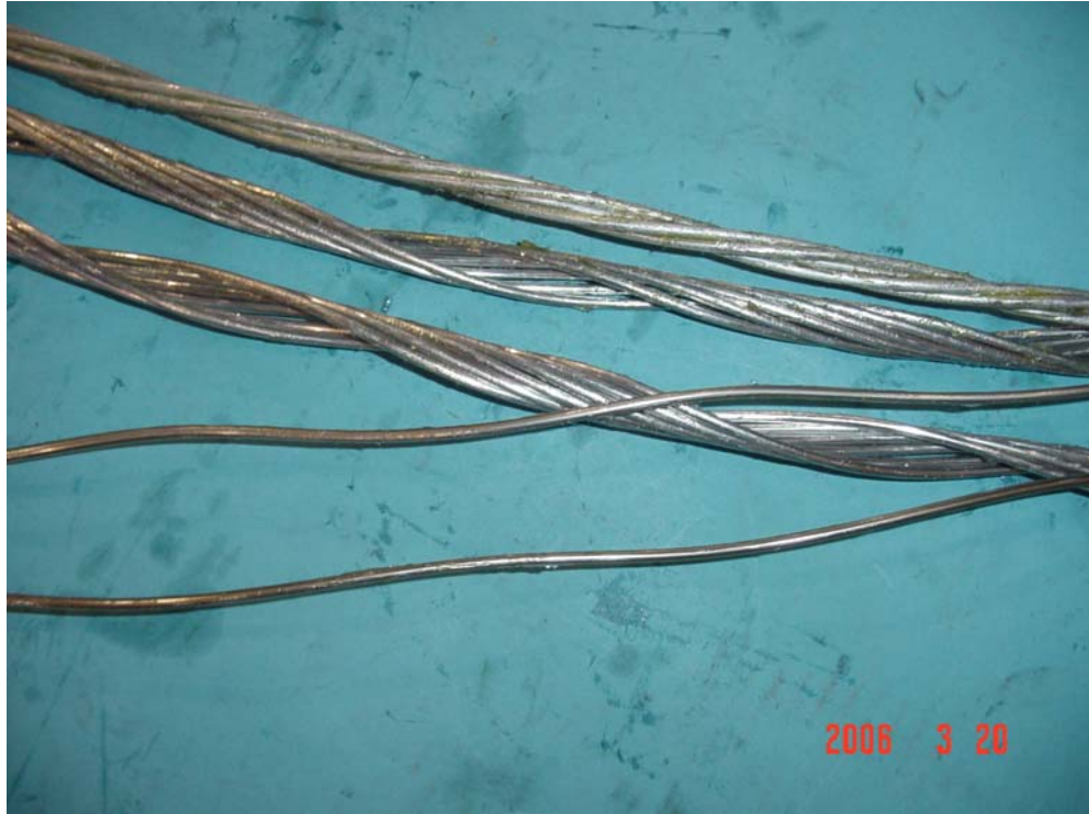
Figure 3a Dissected Components from Aeolian Vibration Test (Under Active Dead-end)
