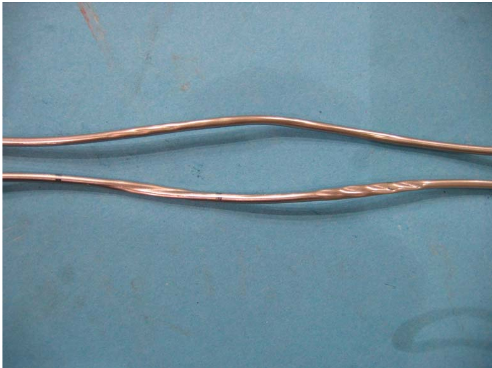
Figure 3b Dissected SS Tubes from Crush test
